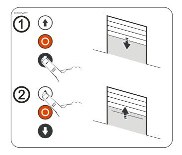
Carry out fine adjustment to correct the OPEN final limit position. Check the door position after correction.
