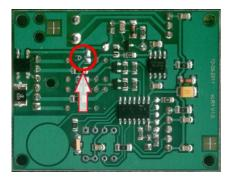
It is possible to supply the eLR1-868S receiver with a voltage of 12V. To do this, connect the solder points marked with the letter "A".
