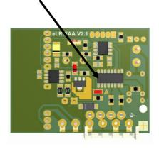
eLRFAA2E/eLRFAA2H with eLA11 module can be used as an independent universal radio-receiver. Open Collector outputs of eLRFAA2 control relays of the eLA11 module.
